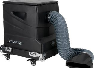
The Entour ICE is a tour-grade low-lying fog machine that creates a thick cloud of smoke that stays close to the floor when used with dry ice. It comes in a road case with casters and features DMX and other on-board controls, a motorized dry ice basket that drops into the water and a low water level sensor that automatically shuts off the pump.
